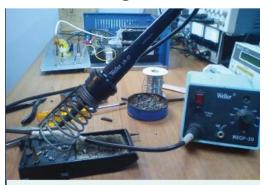
In labs and in many workshops on the campus as well as at home we use desktop soldering irons and tin solder. The soldering process involves health and environmental hazards.
